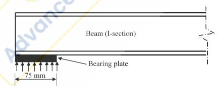
As per IS: 800-2007, the web bearing strength (in kN, round off to 2 decimal places) of the beam is \_\_\_\_\_
