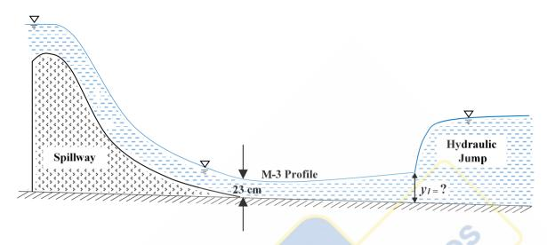
The flow enters as an M-3 profile in the long wide rectangular channel with bed slope =  $\frac{1}{1800}$  and Manning's n = 0.015. A hydraulic jump is formed at a certain distance from the foot of the spillway. Assume the acceleration due to gravity,  $g = 9.81 \text{ m/s}^2$ . Just before the hydraulic jump, the depth of flow  $y_1$  (in m, round off to 2 decimal places) is \_\_\_\_\_\_
